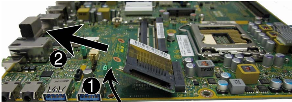
Figure 6-74 Removing the card reader board
